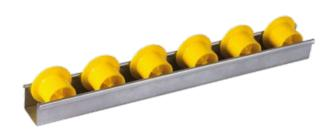
By slightly braking the goods, the mini brake controls the speed on a slope. It is suitable for braking cardboard boxes weighing between 2 kg and 50 kg and is used above all with deep and steep order picking flow systems as well as with automatic systems and different weights of goods. An adapter integrates the mini brake directly into the roller track. The following versions are available: light, light with grip, heavy, heavy with grip and with a diameter of 32.5 mm.
