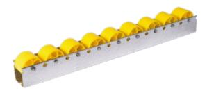
The guide rail, which is particularly sturdy, has a profile width of 1.5 mm and the steel axes are reinforced from 3 mm to 5 mm, which means that they can bear containers weighing up to 80 kg.
