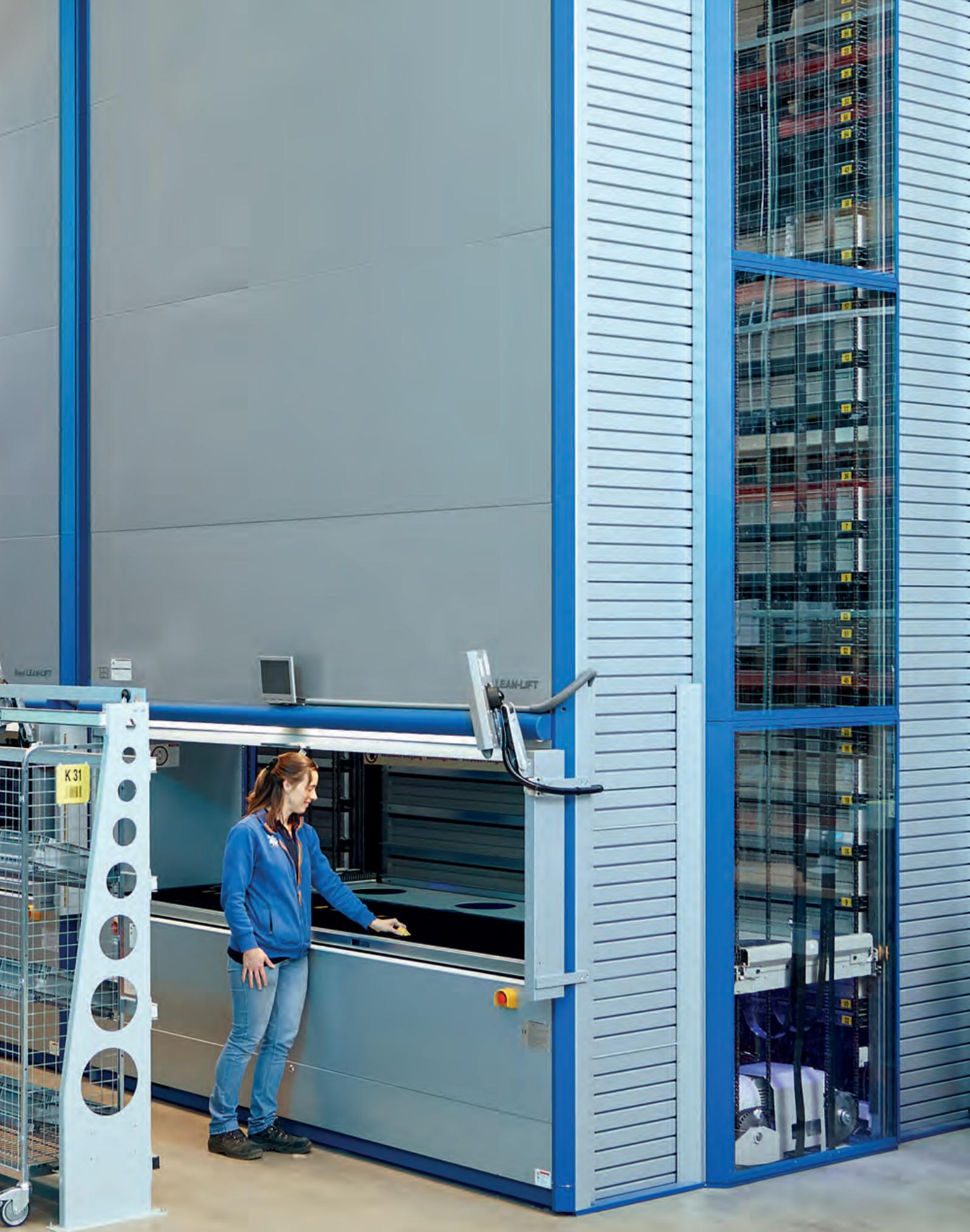
Fast and error-free picking with 12 Hänel Lean-Lift® systems thanks to Pick-by-Light and Drop-to-Light
