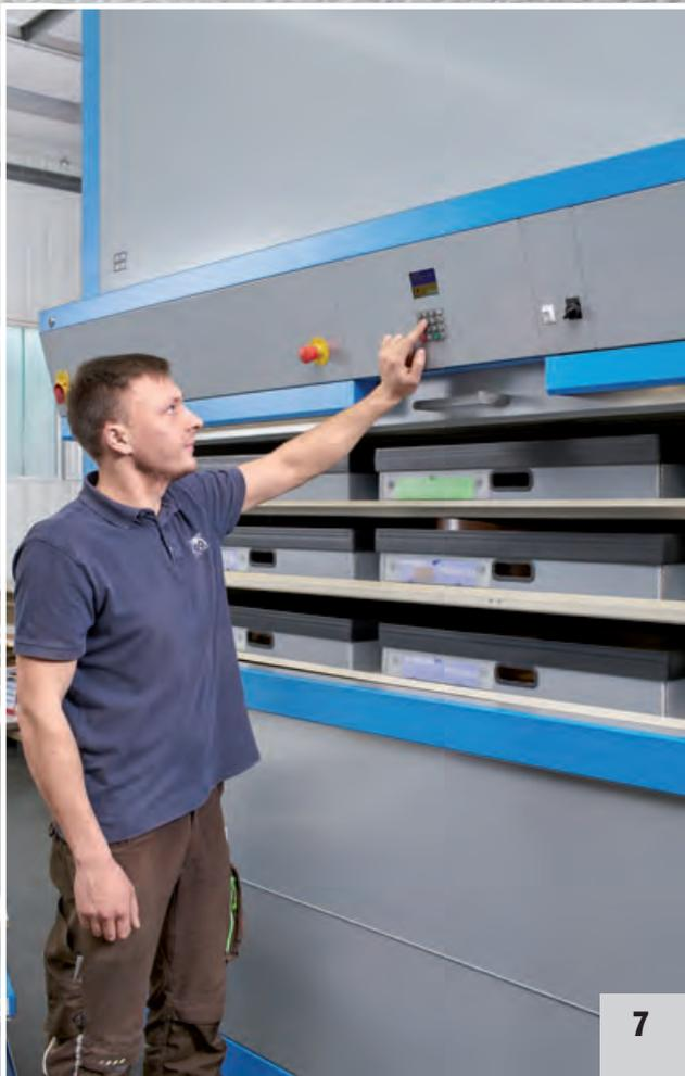
The MPON is integrated in the switch panel above the access point of the Hänel Rotomat® industrial storage system
