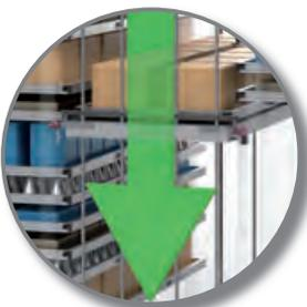
**1** As the extractor descends, electrical energy is fed back into the main power supply
